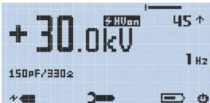
Picture 1. above shows the large touch screen display of the brand new ONYX ESD simulators.
