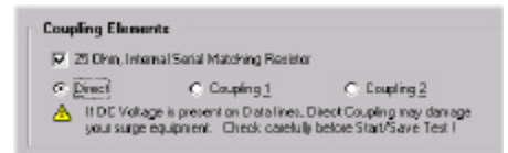
↑ Built-in interactive warnings to prevent incorrect configuration settings which could result in damage of EUT or generators.
